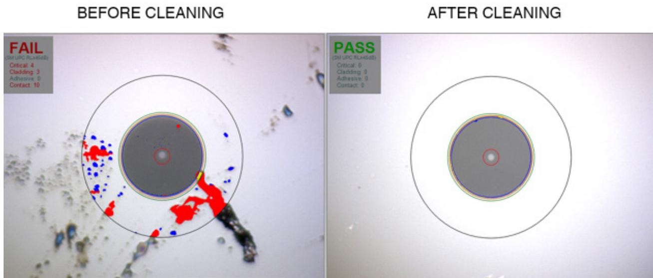
Auto-analyzed images from VIS 400 using inSpec software
