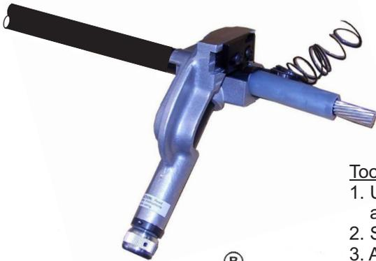
The *Utility Tool* WS9A shaving tool is used to remove bonded semi-con insulation screen from URD cables that are typically, but not limited to cables rated from 5 - 35kv. The tool is applicable to cable with a semi-con diameter of .55" - 2.25" (13.97 - 57.15mm)
